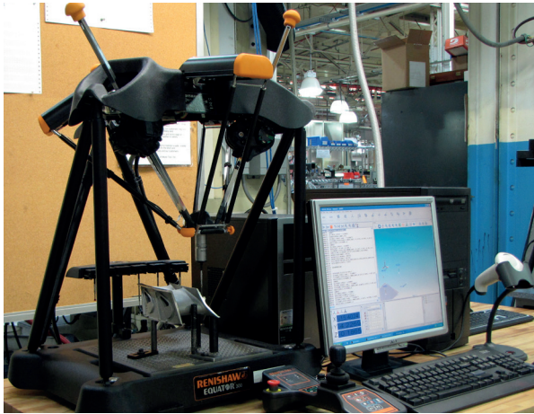
Equator replaces multiple hard gauges and is re-configured with simple programming.
