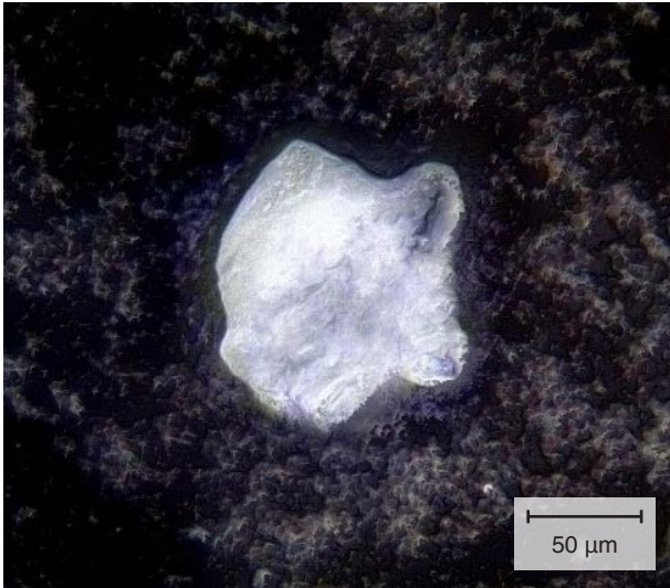
Figure 2: In-focus 2D image of a lactose particle generated using the Z-stack software. The height variation from the surface to the top of the particle is approximately 50 μm. Imaged using a 20× objective (depth of field ~ 3 μm).
