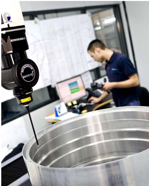
REVO® 5-axis measuring system scanning large bore on an aerospace component.
